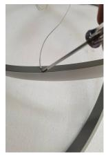
Step 2: Pry open the PVC hood with a screwdriver. Take care of the LEDs during this step, do not touch them.
